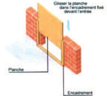
batardeaux (cf schéma), barrières anti-inondation, clapets anti-retour (assainissement), pompe, ...
